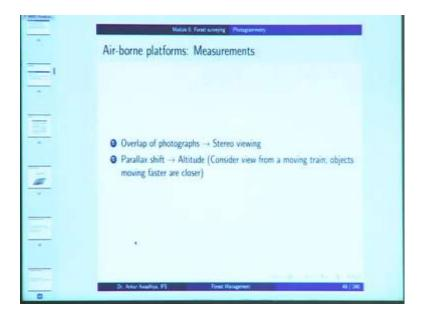
Now, in the case of measurements, you try to take a good overlap, so that you are able to have stereo viewing of the of these different locations, and you can make use of parallax shift to get a an idea of the altitude.
