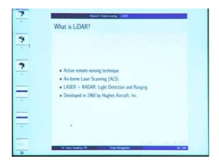
And, in the next lecture, we had to look at LiDAR which is Light Detection and Ranging. It is the word is made from a combination of laser and radar; where radar is radio detection and ranging. So, in this case, this is an active remote sensing technique, in because you are because, you require energy to illuminate the object using the lasers. It is an Air-borne Laser Scanning system or an ALS system, developed in 1960 by Hughes Aircraft.
