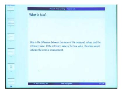
Then, we defined bias as the difference between the mean of the measured values and the reference value. And, if the reference value is the true value, then bias is the error in management in measurement.
