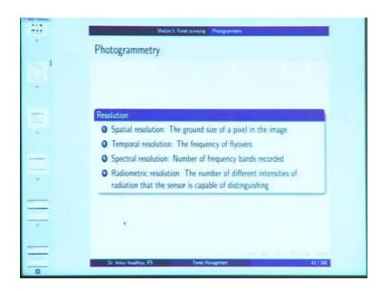
Now, we defined spatial, temporal, spectral, and radiometric resolution. Spatial resolution is the ground size of a pixel in the image; essentially how many megapixels do you have in your camera. Temporal resolution is how frequently are you taking pictures or the frequency of flyovers. Spectral resolution is whether you are taking a black and white image or you are taking a colored image in three different bands or even more number of bands.
