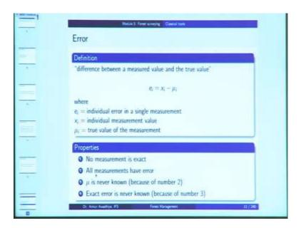
Then, we defined error as the difference between a measured value and the true value. And, the properties are that there is no measurement that is exact; all measurements have some error, and because of this error, you can never know the true value of anything.
