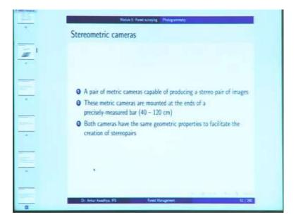
If you want to take stereo measurements, you take a stereometric cameras; in which case, you have to metric cameras that are mounted at the ends of a precisely measured bar.
