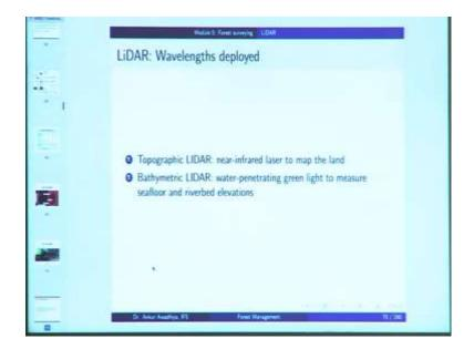
When talking about the wavelengths, you have the topographical LiDAR; in which gives near infrared light laser is used to map the land; or you can make use of bathymetric LiDAR; in which case our water penetrating green light is used, to measure the sea floor and the riverbed elevations.
