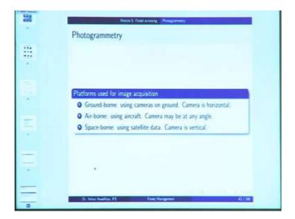
And, in the case of photogrammetry, we typically use three different kinds of platforms. They can be ground-borne platforms, in which case, you are using cameras on the ground. And, the camera is horizontal or you can make use of space-borne platforms, in which case, you are using satellite data, and in this case the camera is vertical. The third option is that you can make use of air-borne platforms, in which case, you use an aircraft or a drone and in this case the camera may be at any angle.
