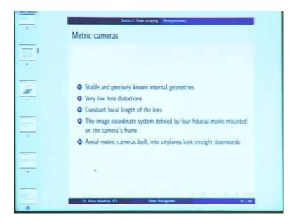
Now, in when you are using photographs to take measurements, it is good to use a metric camera, which is the stable; which has stable and precisely known internal geometries; low lens distortions; constant focal length of the lens.
