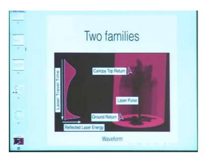
Now, you can make use of a LiDAR in two families; you can make use of waveforms or you can make use of information in a discrete pattern.
