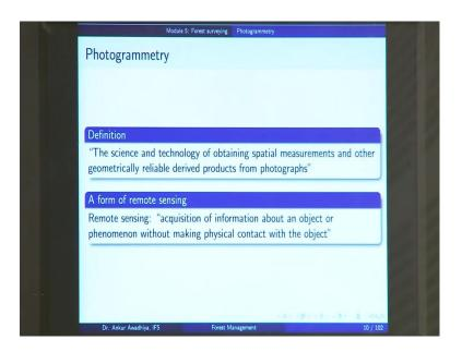
The photogrammetry is defined as, "the science and technology of obtaining special measurements and other geometrically reliable derived products from photographs." So, it is the science and technology of obtaining what? - spatial measurements that is measurements over the space, both in 2 dimensions and in 3 dimensions.
