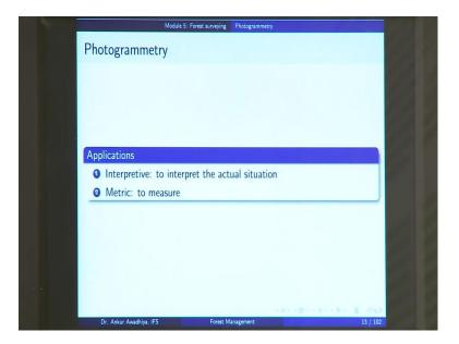
And, there are two applications of photogrammetry. You can use it for interpretation of the surface. So, you can, for instance, if you are doing photogrammetry of a forest area,
