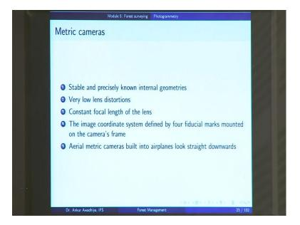
Now, we also make use of metric cameras. So, metric cameras are those cameras that are designed to take the measurements. So, you know each and every thing about these cameras and these are very standardized cameras. These are stable with precisely known internal geometries. There is very low amount of lens distortion, constant focal length of the lens, the image coordinate system is defined by 4 fiducial marks mounted on the cameras frame.
