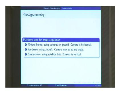
Now, there are 3 platforms that are used in the case of photogrammetry. So, you can make use of a ground -borne platform. So, essentially what this is saying is that you are standing on the ground, and you have a camera in your hand and you are taking different pictures. So, you are based on the ground.
