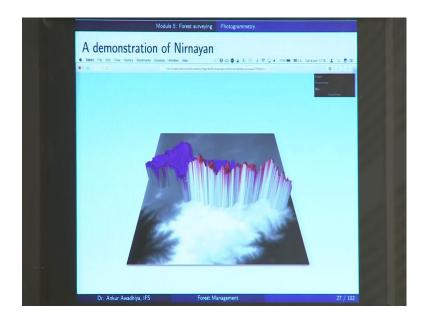
Now, a digital elevation map can also be made use of to give you a 3-dimensional representation of the area.
