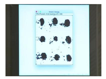
So, in the case of this processing, we increase the contrast of these points, then we converted them into a binary image. Now a binary image is either 0 or 1, and in this case, the dark spots are 0 the bright spots are 1. So, we have converted your image into a binary image.
