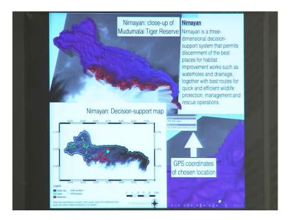
So, for instance, this is a digital elevation map of the Mudhumalai Tiger Reserve. So, in this map, what we are seeing is that what are the elevations of different points on the ground, by making use of the area of the photographs. And, in this case, we are seeing a hydrographical map, where we are saying where are the streams that are located.
