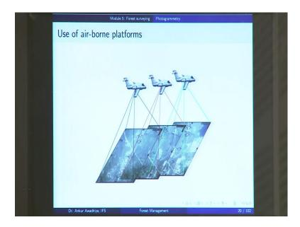
Now, when we are making use of the air-borne platforms. So, this is, for instance, the image of a plane that is moving and then it is taking different photographs. Now, we tend to take photographs, in such a manner that there is a sufficient amount of overlap between each and every of or every corresponding images or every nearby images.
