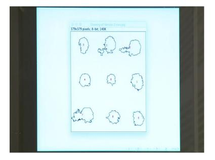
And now, this binary image can be processed in a computer to give you an idea of the number of pits that were dug, and also the area of each and every pit. So, in this case, these numbers were given by the computer. And here, we can see that this is pit number
