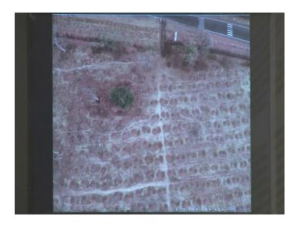
Now, we can also make use of photogrammetry, to say to make metric computations. So, for instance, in the case of this plantation, we can find out whether these I mean what is the distance between these different pits. Now, if you have an idea of the distance between different pits, you will have an idea of the density of the plantation, and you will also have an idea of whether there will be in overcrowding in this plantation or not.
