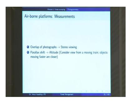
Now, take to take measurements, you require two things: one is that you require overlap, so that you are able to have a stereo viewing, in which case you are able to see a 3 dimensional view of the object, and you also make use of parallax shift to discern the altitude.
