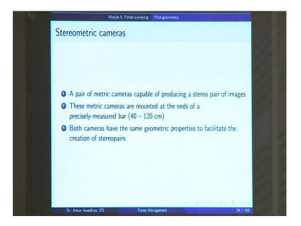
At the same time, so, so, we also make use of stereometric cameras, in which case, you have two cameras; so, stereo image is anyways, in which case, you have two cameras that are taking the image, and stereometric camera is two metric cameras that are being used. So, it is a pair of metric cameras capable of producing a stereo pair of images.
