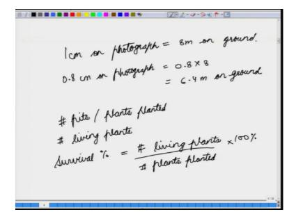
And once, you have that scale that 1 centimetre on photograph is equal to say 8 meters on ground. Now, you can make use of this information, and suppose the pits are at a distance of say 0.8 centimetre. So, 0.8 centimetre on photograph in that case will be equal to 0.8 into 8 is 6.4 meters on ground. So, what we are using photogrammetry in this sense is to is to use it for a metric computation.
