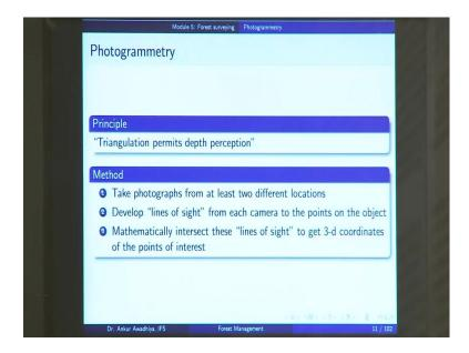
The principle that it uses is triangulation. So, in the process of triangulation you are able to perceive depth. Now, what is that mean? So, for instance, you are looking at one object and you are looking at it from two different points.
