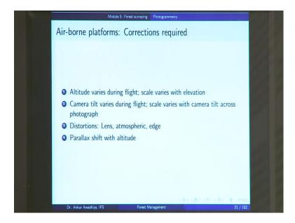
Now, when you are making use of air-borne platforms, you need to perform certain corrections to the image the if the altitudes varying according to the during the flight, then the scale is varying with a elevation. Because if you are looking at things from a greater distance, then they appear smaller in size. So, the scale is different as compared to when you are looking at the images or looking at the objects from a closer distance.
