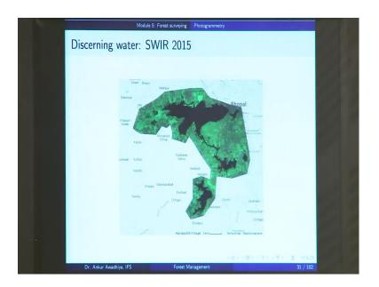
So, we can get these transition classes, but to make the boundary we can also make use of things such as the shortwave infrared bands. So, this is an image in the shortwave infrared band. Say for every year say 2015, we can make an image like this, from which we can get where the water is located by making use of the normalized difference water index.
