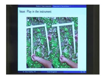
Also, in a number of instruments you have a certain amount of play in the instrument. What do we mean by play? It means that this moveable jaw which should be at 90 degrees to the main axis - it is either inside or outside, or it can even swing.
