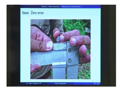
A number of these instruments also have zero errors, which means that when you bring both the jaws together they do not match at the zero point.
