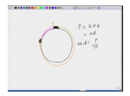
So, if you have a tape, it is difficult to measure the diameter directly, but what you can do is that you can put your tape all around this your trunk, and get the value of P, which is the perimeter.
