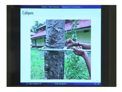
So, how do you take the measurement? You put the caliper in such a way that your tree is coming between the fixed jaw and the movable jaw. Then, you move the moveable jaw such that it, such that both the jaws are able to touch your tree at the designated breast height, and then you take the measurement directly from the scale; that is easy, but then there are also certain issues.
