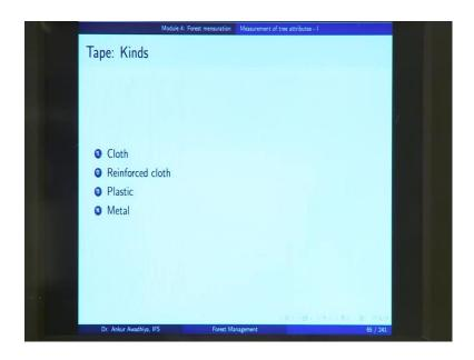
Tapes can be of different kinds. you can have a tape that is made out of a cloth. This cloth may be reinforced, especially with metal; so, that its life increases. You can have a plastic tape or you can even have a metal tape. So, there are these four common kinds of tapes.
