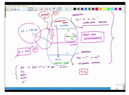
So this is how it looks like, so you have the valence band sitting here, you have the conduction band sitting here and you have the light which is falling out here, the h mu as we talked about less than 300 nanometer 390 nanometer, so here you are having the holes which are positive deficiency in electron and you are having the electrons ok and this is your conduction band whereas this molecule is your valence band ok.
