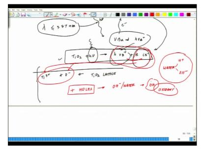
So in titanium oxide if you remember when we talk about retile, we talk about it is a band gap of 3 to 3.2, it has 3 polymorphs and they vary from 3 to 3.2 electron volts ok. So the light energy what has to be provided in photo catalysis light of energy greater than the band gap of a semiconductor. So the light energy h mu has to be greater has been light energy has to be greater than 3 to 3.2 electron volt ok.
