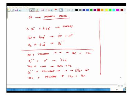
So this was one powerful oxidant because we are generating ROS reactive oxygen species. Similarly the hydroxyl radical can subsequently be oxidized OH could subsequently be oxidized ok, because can subsequently oxidized the organic species. So this is when you talk about the organic pollutants or any other stuff oxidized organic species with mineralization producing mineral salt like Ceo2 and water ok.
