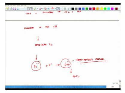
And if you look at it there is series of reactions which are happening here and these are and these are just a handful of them. So electron in the conduction band can be rapidly trap by the molecular oxygen, so electron in the conduction band could be rapidly trap by the molecular oxygen adsorb on the titanium particles which is reduced to form superoxide radical which is O2.- ok.
