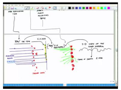
So, here is your sample, these are area of atom sitting out there and 1 more thing you forget to mention is when you do TEM or transmission electron depending on the kind of particle out here. You may be able to see the surface of the particle with the electron density pattern which we call as the frinze lines you can observe this in a pictures when if you see a transmission electron microscopy picture with there is see the frinze lines.
