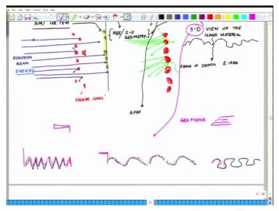
The way it works AFM, so AFM is one beautiful surface characterization technique say for example I have a surface like this drawing the surface a pattern depth surface or a surface like this. If you see the distinct feature of the 2 surfaces or surface like this what I do I take a probe like this, just imagine a probe which can really travel through it. So, this probe is travelling on the surface like this, it stopping on the surface and it is moving.
