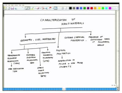
So, as I mention the characterization could be separated in 2 categories, 1 is characterizing the geometry, size and also we can call it morphology whereas the other set of characterization includes your surface chemical properties. I use the word surface chemical because when we talk about nanomaterials we talk about dimension which is maybe 1 atom or 2 atom thick.
