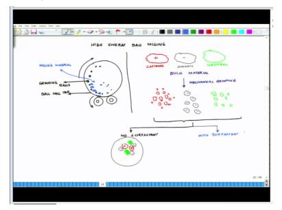
So, high energy ball milling, this is the very first technique okay, so high energy ball milling essentially what happen is that. Say for example you have this grinding ball which is moving in a particular direction and this supported by other small balls are there in this okay. So there is a grinding action which is happening which could you see out here okay and this is this whole thing is moving and inside it you are having the grinding balls.
