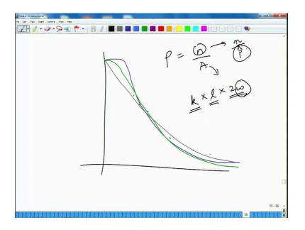
So, essentially when we have some points, we could fit a model say like this. A negative exponential model or we could say that we are going to fit a hazard rate model something like this or we could say that we are going to fit a half normal model something like this.
