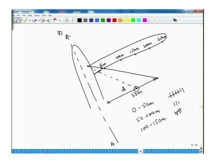
Now, in an aerial survey you have any aircraft and on the wings we have put some struts. So, the struts are basically distance estimators. So, we can just say that this is say 50 meters, this is 100 meters, this is 150 meters, this is 200 meters and this is 250 meters.
