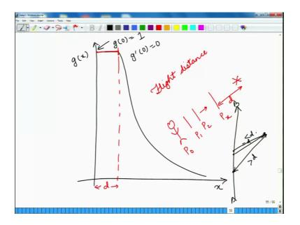
Now, we can understand a hazard rate function by looking at its shape. So, the hazard rate function has a broader shoulder as compared to half normal and then it goes down with distances x. What do we mean by this shape? It means that at g of 0 we have it as 1 and g prime of 0 is 0.
