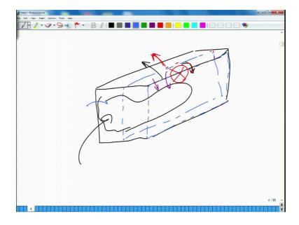
So, what happens in this case is that you have, so, if you are looking it from the other side. So, we have. So, this is our cage for a squeeze cage. And then we also have another wall that is here. Now this wall which is also made out of steel is moved by the operation of a wheel here.
