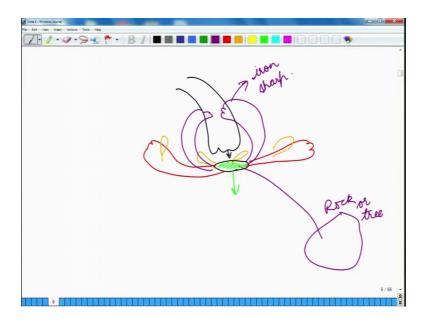
So, this is how the trap would be set up out there in the field. We might even put certain amount of leaf and other litter on top of this trap to conceal it. Now when an animal comes and puts its paw on top of this release mechanism, so, this is to say this green colour is our release mechanism.
