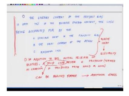
That the energy content of the product gas the energy content of the product gas is up to 75% of the biomass energy content of the biomass energy content okay the loss being accounted for so where are we having the loss the loss being accounted for laws being accounted for by the sensible heat in the product gas either a by the sensible heat in the product gas one way.
