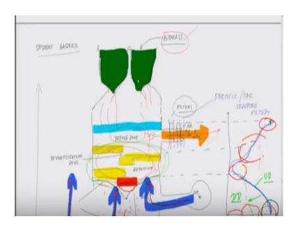
Okay so we talked about the six bit gasifiers as I told you it's a very traditional process and functions at around thousand to know 1400°C I they could see and it is classified under up drift system where the air is coming from bottom and going up let's again look at it ok here is coming from bottom and going up the next arch and the by the way in the up drift the gas which is coming out.
