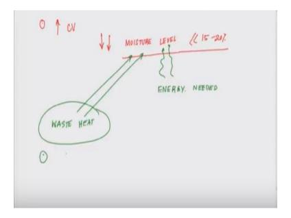
Okay next important aspect is how one can increase so this is a challenge how you can increase the CV order calorific value so one approach is that you have to reduce down on the moisture level. So reducing the moisture level to something less than 15-20% is a challenge but as few people remember in the last class at the very moment you wanted to do this reducing moisture level.
