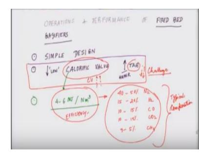
Okay operation and performance of six bed gasifier operation and performance of fixed-rate gasifiers okay so the first point to remember out here it's a very simple design and this is the very first one which were utilized by mankind simple design there is no complexity by this time must have seen so you have the feeder you have the drying zone you have the combustion zone any of the airflow and you have a collector and you have a gas output.
