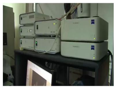
So for this I have used this live cell imaging whole facility and for this we can use this is a chamber where we keep 35mm glass bottom dish inside this and then we maintain temperature and CO2 via these modules and humidity as well by setting all the parameters and then we can maintain all the parameters and we visualize what happening in the inside this cell.
