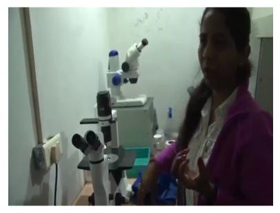
Student: Apart from this life cell imaging we have to other microscopes as well. We have one as inverter one and other one is stereo microscope or you can say it is a dissecting microscope so this normally we use to dissect our minute like a brain dissecting brain from the mice embryo and this we use to visualize cells morphology.
