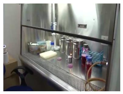
So here is the facility so as you can see here you have a room which is secluded and you have what is called as a bio safety cabinet this is class two like cabinet we are in you know the air that is thrown in t the cabinet is sterilized and then again it gets into and gets filtered so you can see
