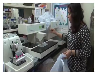
Student: So this is the wax station that we have we for historical analysis we embed the tissue in this tissue embedded as we can see it has. The tissue amyloid is very soft so we need to invade in a system where we can easily process them for cutting out the thin section like we as we know that we need 5 to 10 micro metre of sections for seeing the historical genesis in that.
