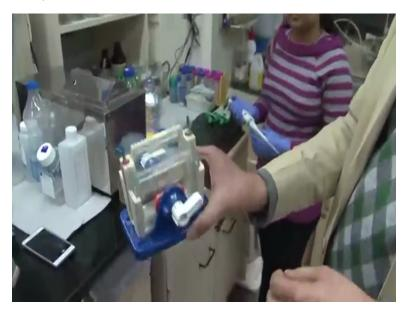
So why don't you show this (())(07:55) so this an apparatus wherein you can (())(08:00) for what you call as (())(08:02) so these are very thin gels which you can use to separate for example protein or oligonucleotides or DNA RNA that are very very small in size in bases 100, 50 bases 100 bases and so on so that is what she is setting up this is (())(08:19).
