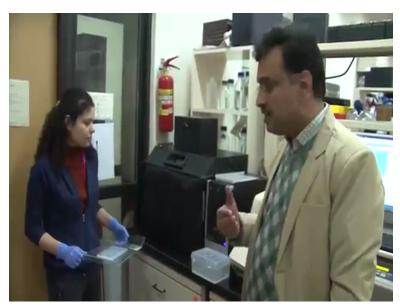
Professor: So basically this is an instrument which has a UV box which so transilluminator what you call, so when you staining the DNA, RNA with certain stain for example ethylene bromide
