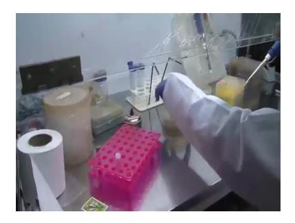
Komal again working using class-1 laminar flow in which the (())(18:06) taken in and you have filter that sterilize the air and throws it out via this this area therefore the chamber within is clean and she is doing an experiment where she is trying to clone it and what you see around are bacterial dishes and Komal why do you not explain.
