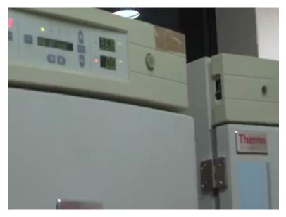
Professor: So these are the what you call as a incubator so basically these are the machines that maintain the temperature 37 degrees not only that it also maintains the carbon-di-oxide ok that is to make the medium PH maintain.
