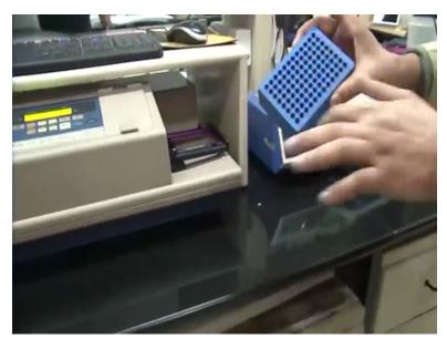
Professor: Right so that that is one application likewise we have again a high through put machine this machine has you know plate this called as a micro, plate (())(05:46) which is a 96 (())(05:48) so it has 96 for example you can you know have you know test tubes or small tubes
