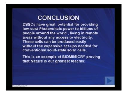
And this is the classic example what is believed as you know as a case of Biomimicry dye sensitized solar cell have the great potential providing low cost photovoltaic power to billions of people around the world living in remote areas without any access to electricity. These cells can be produced easily without expensive set-ups need for conventional solid-state solar cells.
