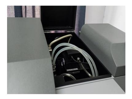
So, this is the chamber where you place your cuvette. The cuvettes used for CD spectra spectroscopy are quartz cuvettes because you are working in the UV range and glass strongly absorbs the UV radiation. So, you need quartz.
