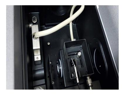
This is the cuvette chamber. So, what you are seeing here these are the adapters which I am taking out right now. You can see them. So, once you take out the adapters you will see that you can easily fit a 1 centimeter path length cuvette in this sample chamber. A 1 centimeter path length cuvette is generally used for near UV CD which is weaken
