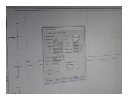
So, generally when you record CD spectrum you record two channels. Channel 1 is CD and Channel 2 is High Tension HT voltage. We can set up the wavelengths here we will be recording the CD spectrum from 250 to 195 nanometers. This is the far-UV region where absorbance is largely because of the peptide bond.
