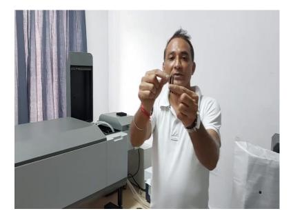
So, you have these two adapters. You place them in the cuvette chamber and you simply sandwich your 1 millimeter paths and quartz towards between them and put it here. The volume of the 1 centimeter pathway towards cuvette is roughly around 200 microliters; that means, you need 200 micro liters of sample for doing the five UV CD spectroscopy, ok.
