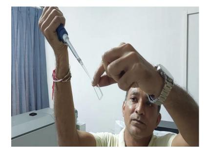
This will be our blank. You add the blank or whatever sample you are adding to the edge of the cuvette ensuring that no bubbles enter inside the cuvette. So get the cuvette and gently push down the solvent ensuring that no bubble enters in the cuvette. You can gently tap the cuvette to get a nice meniscus on the top.
