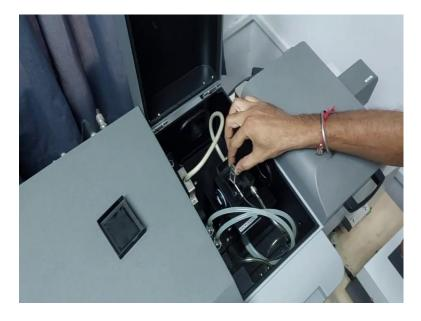
We place this cuvette now in the sample chamber like this. Cover the sample chamber, close the lid.
