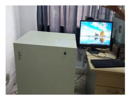
So, with this CD instrument we also have a nitrogen generator which will filter out the oxygen from the atmosphere and generate nitrogen. So, you can flush that nitrogen gas through the instrument and then only you turn on the lamp of the instrument.
