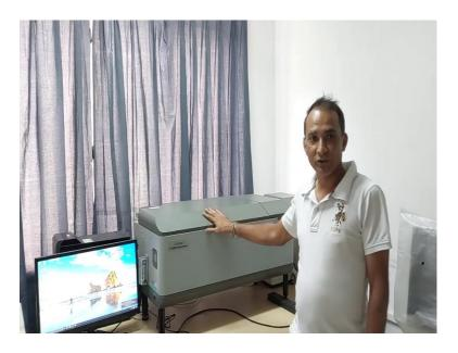
Welcome to the demonstration of CD spectrometer. I am Doctor Nitin Chaudhary a Professor at the Department of Biosciences and Bioengineering IIT, Guwahati. This is CD spectropolarimeter from Jasco and this is what we will be using for recording the electronic CD spectrum for some proteins or peptides. A far-UV CD spectrum is mostly used for studying the secondary structural elements in a protein or peptide sample.
