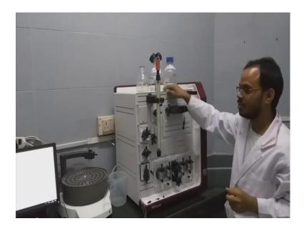
So, what we will do we have to change this pumps into water. So, we changed into water. Now, we can connect to the column. Here also some of the precautions needs to be taken. If you are using chilled buffers ok suppose you need cold buffer. So, that means, you have to bring those all the components of the system to the temperature which you want to use for your purification.
