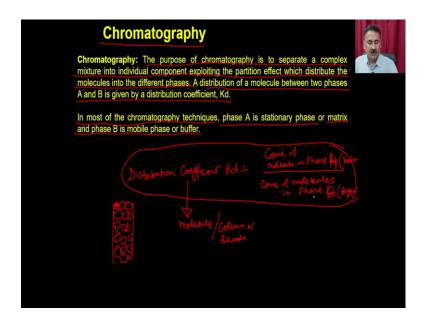
Now, what is chromatography? Chromatography, the purpose of the chromatography is to separate a complex mixture into the individual component exploiting the partition effect which distribute the molecule into the different phases. A distribution of a molecule between the two phases A and B is given by the distribution coefficient. So, distribution coefficient is distribution coefficient Kd is equal to concentration of molecule in phase 1 divided by the concentration of molecule in phase 2, ok.
