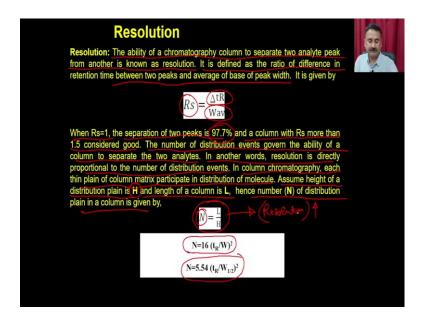
So, resolution is the ability of a chromatography column to separate two analyte peak from another and it is known as resolution. It is defined as the ratio of difference in the retention time between the two peak and average of the base of the peak, which means the resolution is directly proportional to the difference between the two peaks and it is going to be inversely proportional to the average of the base of the peak.
