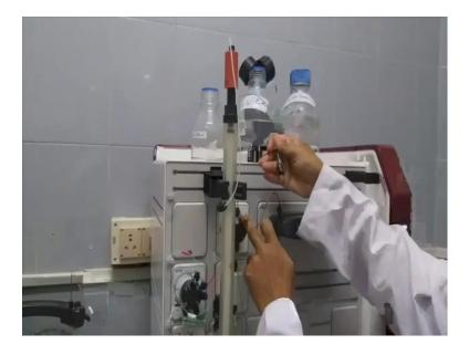
So, here this is the software system flow I am keeping 0.5 ml per minute since we are going to connect the column. So, if the flow rate is more then the pressure alarm may come. So, after that we have to set the monitors. So, this is also I am going to set system flow 0.5 insert and now we have to set alarms.
