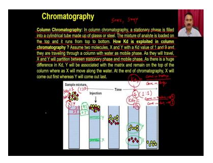
So, how the chromatography is separating the molecules? So, column chromatography in a column chromatography at stationary phase is filled into the cylindrical tube made up of glass or steel. So, this is the cylindrical tube where you have filled the beads right they can be made up of glass or steel. The mixture of analyte is loaded onto the top and it runs from the top to bottom.
