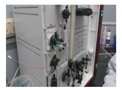
So, for injection purpose this is the port where we are going to inject the solution protein solution and this is the loop Whatever we inject through this injection value it will be stored inside the slope. The size of the loop depends on how much protein you want to inject and the column capacity.
