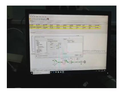
And we can see there completely flat line flat signal corresponding to UV 280 So, that means, there is no ethanol inside the column. In addition to that we already washed 30 ml of water. So, the total column volume inside the column is it is around 25 ml. So, we also washed with 5 ml extra. So, we can be sure that it is completely removed.
