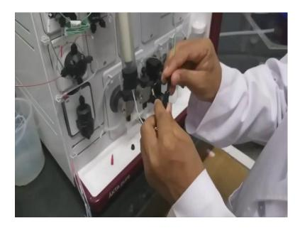
Once you see the buffer filling in you just have to connect with the downward portion. So, now the column is connected to the system and you need not to touch anything everything will be operated on the software.
