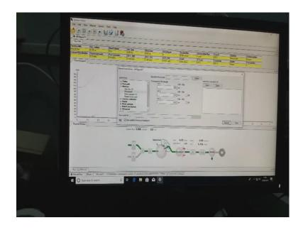
So, this will give different we can change a different commands using the software just go to manual execute manual. So, this is the manual instruction software or dialog box where you can change things. So, here different parameters you can change through this pop-up window like pumps flow path and various parameters such as monitors next to go to pumps.
