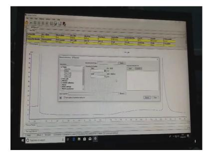
So, in main system control here fraction collector there is a option for fraction collector. How many fractionation you need to be done when you need to stop fractionation and how much feed to fractionation outlet wall all these things you can set there. In addition to that you can also set system gradient flow.
