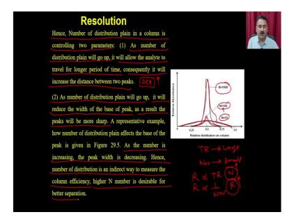
Now, hence the number of distribution plane in a column is controlling two parameters and how the resolution is getting affected by the number of distribution plane. Because as the number of distribution plane will go up, it will allow the analyte to travel for a longer period of time.
