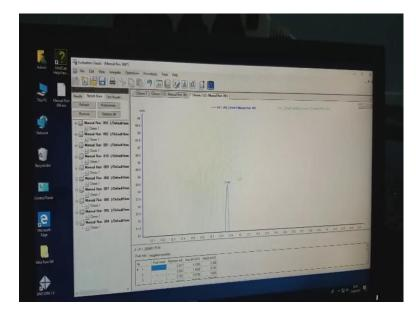
So, here we can see 12.86 this is the major peak what we have. So, with this you can analyze the results. So, if you want to calibrate you have to calculate retention volume for all the proteins whichever you are using for calibration and construct the calibration curve between partial coefficient and lab molecular weight.
