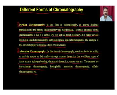
Now, we have the different forms of the chromatography you can have the partition number 1 you can have the partition chromatography or number 2 you can have the adsorption chromatography. In a partition chromatography in this form of chromatography an analyte distribute themself into the two phases, liquid stationary phase and the mobile phase.
