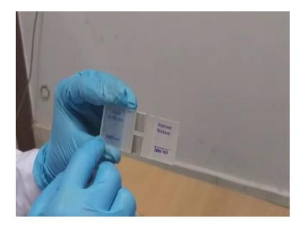
Before counting, we have to see how a counting chamber or hemocytometer look like? This is a typical hemocytometer also called as Neubauer chamber which contains these squares in upper side and lower side, with each square having depth of 0.1 mm and area of 0.0025 millimeter square. Now, I am going to put a cover slip on this chamber then I will add slowly cell suspension through capillary action it will spread all over the squares.
