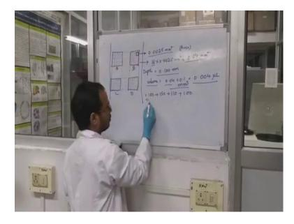
So, we checked how many cells are there in all the squares. Now, we have to count how to count the cells. So, here a typical Neubauer chamber which contains squares, 5 squares. So, we have to count cells in these squares. So, each square is an area of 0.0025 millimeter square and total small squares 16. So, total area of this whole square is 0.04 millimeter square.
