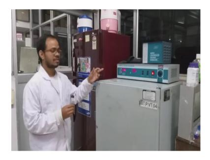
So, it should be 37 degree Celsius and 150 RPM. Now, we can see some growth in here. Now, we have to check what is the OD of this culture. We can measure it in spectrophotometer at 600 nanometer Now, how to take out one mm from this culture and plank against the media and at the (Refer Time: 31:29) you have to measure the cultures. I am going to use spectrophotometer to measure what is the OD of the bacteria. Now, before doing that, I have to plank against the media. So, this is the plain media.
