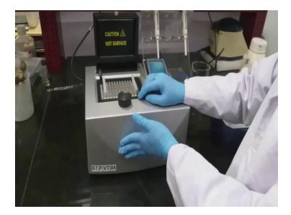
This is an earlier version of thermal cycler which contains display unit where we can observe the parameters and change the parameters. This is the hot shield, this is sample holder, and inside there is a Peltier system which can maintain the temperature fluctuations.
