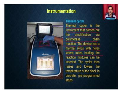
So this is what you are going to see, this is actually a thermal cycler, where you are going to have the, a block where you actually can be able to put the reactions, and a thermal cycler is an instrument that carries out the amplification by the polymerase chain reactions. This device has a thermal block with the hole where tubes holding the reaction mixtures and these cycles can raise and lower down the temperature of the block as per the programming.
