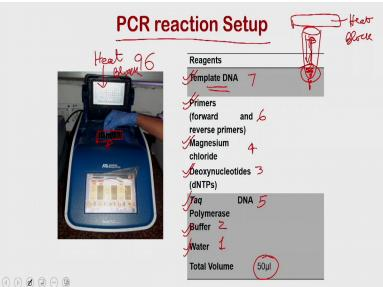
So this is what the PCR reactions, this is the PCR machine, typical PCR machine what you have is the heating block where you are going to setup the reactions. So in this heating block you have the place for keeping the Eppendorf. Normally you have the 96 places for keeping the reactions. And on the top of this, you have a heat block; this heat block is being placed on the top so that when you heat these reactions from the bottom it should not going to evaporate the sample.
