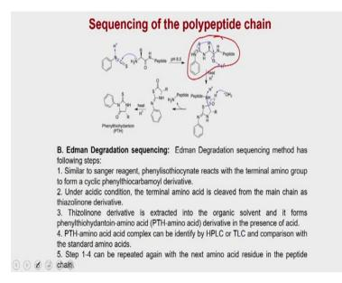
So this is the Edman Degradation Method. So Edman degradation method also we have discussed and the Edman degradation method similar to the sanger reagents. The reagent is very different but the overall working principle and other things are very very similar kind of thing. Where you actually are making adduct with the terminal (phospha) terminal amino acid and this adduct is what you are characterizing in the Edman degradation method also.
