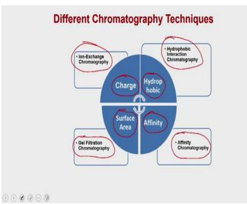
So that is what we have decided. So if the protein is having a charge you can actually use the chromatography technique that is called as the Ion Exchange Chromatography. The protein has the hydrophobic patches. Then you can use the chromatography technique that is called as the Hydrophobic Interaction Chromatography. If the protein is having a different surface area or the hydro dynamics volumes then you can use the Gel Filtration Chromatography.
