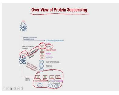
After this we discuss about the sequencing techniques. So in a typical sequencing technique what you are doing is, you are actually cleaving the proteins with the help of trypsin. First you are, first you are removing the disulphide bonds then you are cleaving the protein with the trypsin
