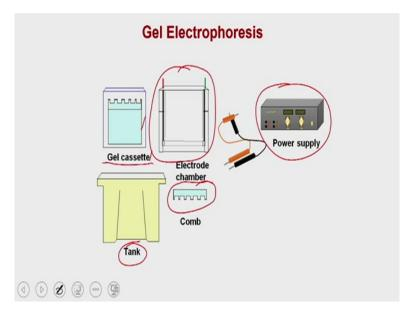
Vertical gel electrophoresis has multiple components such as the gel cassette. You have the electrode chamber, you have the power pack or the power supply unit. The purpose of the power supply unit is that it will allow to run the supply current of the positive or the negative charges, then you have the tank and then you have the comb to prepare the wells and you also have the gel cassette, so that you can be able to cast the gel of your choice.
