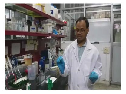
So this is the glass plate. This is very thin one, so this is the main glass plate this is 1.5 mm glass plate. It is available in 1 mm glass plates also. If your loading solution is less like you want to load only 20 micro-litre, 30 micro-litre then 1 mm gel is good enough, but if you have extended volumes like 70 micro-litre you can use 1.5.
