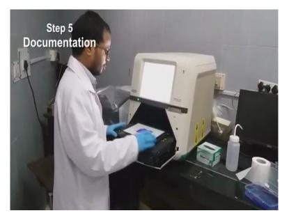
Now, we will capture the gel image. So you can see manually also but for record purpose we have to capture it through gel doc. So this is the gel doc imaging system from (())(65:37). So I will show you how to capture images. So here we will use the white tray. There is another one grey or UV tray is also there.
