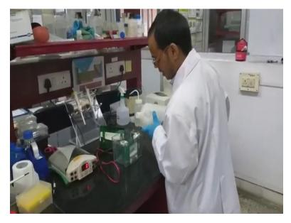
Once fixing here we have to add this running buffer. The running buffer contains 15 grams of Tris, 72 grams of glycine and 5 grams of SDS for 2 litres of solution, 1x solution. So this is 1x I already prepared, I am going to add. We added in this tank but the main tank surrounding to this one, we have to add up to the mark.
