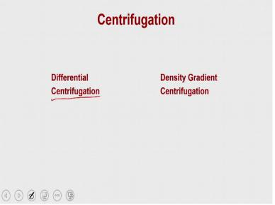
You have the differential centrifugations or the density gradient centrifugations. In the differential centrifugations what you do is, you run the sample at different speeds or different RCF values and because of that, when you spend down, the molecule which is corresponding to that RCF value get pelleted down and you will find that particular organelle or the substance in the pellet fraction whereas the supernatant will contain all other molecules.
