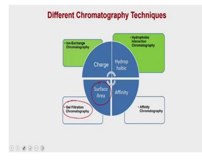
Now, before going into the details of the Gel Filtration Chromatography let us discuss how we can exploit the surface area of a protein to characterize the particular protein as well as how that can be used to purify the different protein from a complex mixture.
