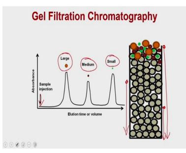
So, this is what we are talking about. If you resolve the molecules of different sizes if you inject the molecule, what you will see is the large-sized molecule will come out first, the medium-sized molecule will come out later and the small-sized molecule or the smallest size of a molecule will come later which means the elution volume for the large is going to be very small.
