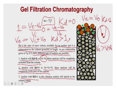
So, that is the formula for K d. So, K d is the ratio of inner volume available for an analyte, is the independent to the column geometry or the length. As per the relationship, three different types of analyses are possible in a gel filtration column. Now, imagine that you have an analyte which has a K d equivalent to 0, K d is 0. If the K d is 0 if you put the0, then what will happen is that V e minus V o divided by V i.
