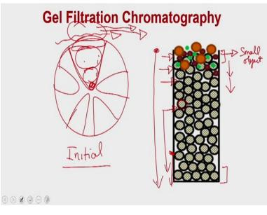
Now, let us understand so what is the kind of pore is present and how the separation is occurring in a gel filtration chromatography. So, if I show you a pore this is the gel filtration bead and the pore is present in a funnel shape pore which is present on these beads. So, you can imagine that you have a funnel shape beads which has a pore-like this from all the sides.
