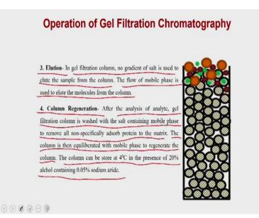
Now, once you have done you can do the elution, so compared to the ion exchange chromatography or the hydrophobic interaction chromatography in gel filtration there is no gradient of salt to use to elute the sample from the column. The flow of the mobile phase is used to elute the molecule from the column. Once you are done with the elution you have to
