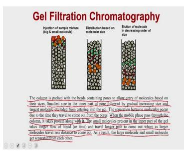
Now, let us understand how the gel filtration chromatography work. So, in this particular chromatography, the column is packed with the beads containing the pores of different sizes and that is going to resolve or going to allow the entry of molecule based on their sizes. So, you can imagine that you have injected a complex mixture of the protein molecules which are of different diameters of like orange, green, red and so on.
