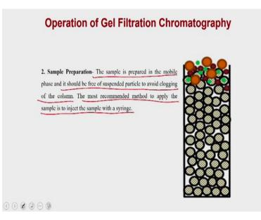
Now, once the packaging is over then you can load the column and you can prepare the sample in your mobile phase. So, whatever the condition of your mobile phase you can use and you have to ensure that it is free of suspended particles so that the column is not going to be clocked. The most recommended method to apply the sample is to inject the sample with a syringe.
