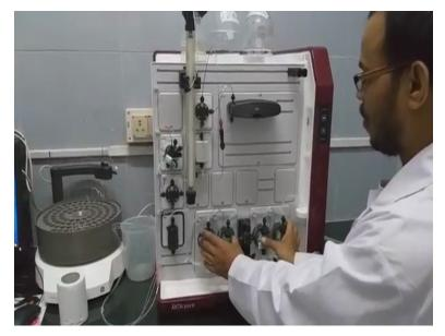
So these two are pumps this one pump and two pump this two sets. Whatever buffers are coming from this buffers tray it will enter here okay these pumps whatever the pressure they are getting they can be embedded here this is the pressure monitor. So once he pressure is monitor it will go to for mixer.
