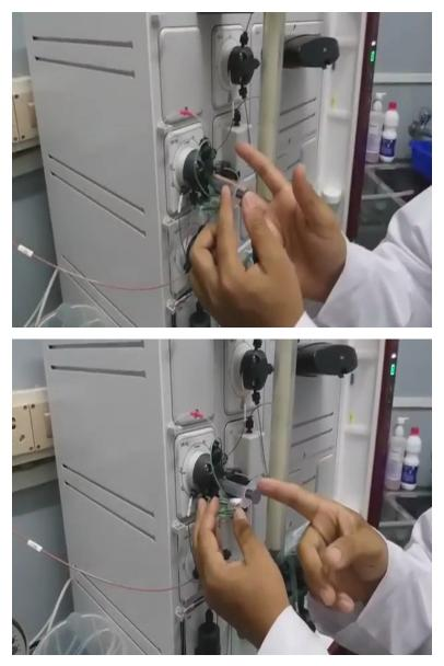
So for injection purpose this is the port where we are going to inject the solution protein solution and this is the lock. Whatever we inject through this injection (())(29:42) it will be stored inside this lock. The size of the lock depends on how much protein you want to inject and the column capacity. So we have 13 reduction column also it can be used up to we can inject up to 1mm.
