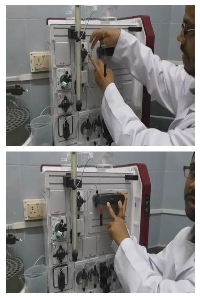
So once it entered in let loop it will go to this chamber it can be connected to the column. So the top portion of the column it will connect here we will show you how to connect the column in coming video. So after that whatever it comes it will enter here and it will come directly into the UV chamber were the eluted component will be detected.
