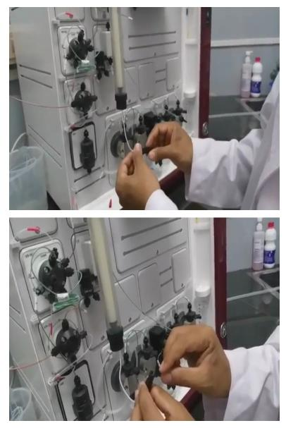
So next here this is the column-connecting portion. So, where her this is the upward portion we have to connect with the column now we are not using column so just we have to go to the column we just click this one column done. So from top to bottom now you can see highlighted one. So you cannot directly connect to the column first you have to fill the buffer or water in this loop. So that there is no air bubbles just open upside of the column with the buffer itself you just directly connects.
