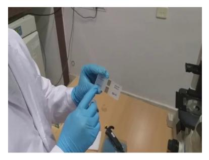
This is the typical hemocytometer also called as neubauer chamber which contains this squares in the upper side and lower side. With each square having the trough point 1 mm and area of 0.0025 millimeter square. (Refer time slide: 31:02)
