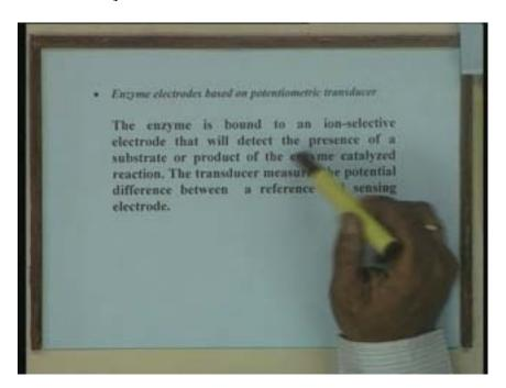
The transducer measures the potential difference between a reference and sensing electrode. We are not doing any manipulation with the transducer; we use the commercially available transducers. It could be a ..... electrode what you use in the fermentor for measurement of dissolved oxygen because that is amperometric transducer; it measures current. On the other hand a simple pH meter or an ammonium ion electrode or carbon dioxide electrode they are potentiometric transducers.
