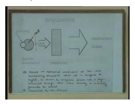
In the electrical circuit current is a very easily measurable parameter and just to make it suitable for repeated use we need to immobilize the bio element. Theoretically the system can be used in a soluble form also but just to make it a continuously usable system the bio element is immobilized.
