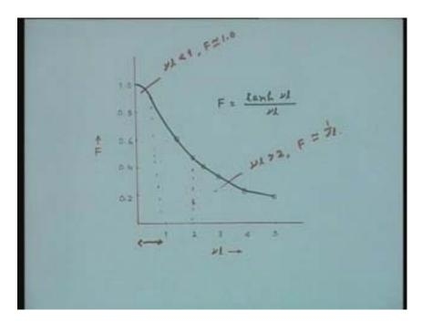
When you say F is equal to one, there is no effect on the kinetic parameter  $K_m$  or there is no diffusional limitation in other words. The  $K_m$  is not altered as a result of mass transfer, diffusion. F is equal to one and as we defined earlier  $K^{app}_{\ m}$  was equal to  $K_{\ m}/PF$  and P we have considered as a constant parameter as far as the immobilized enzyme preparation is
