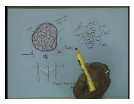
I like you to have a look at the substrate gradient. If you consider that this regime is the thin film then from the bulk there might be a linear substrate gradient across the thin film and the concentration might drop at the surface and from the surface to the interior of the particle that means to center of the particle there might be again a gradient as a result of biochemical reaction.
