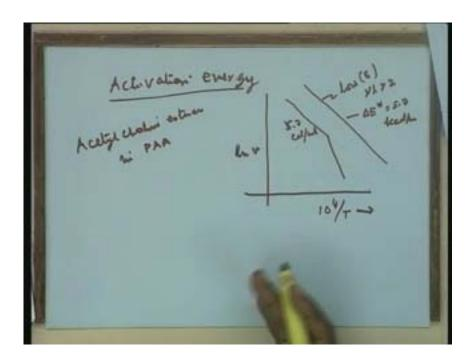
At high temperatures these similar activation energy was obtained even at high substrate concentration as in the case of low substrate concentration because at high temperatures the reaction rate was high. The reaction rate being high, the diffusion became limiting. The activation energy behaviour was almost similar as in the case of low substrate and at high  $\gamma$ l which was established parameters for diffusional limitations.
