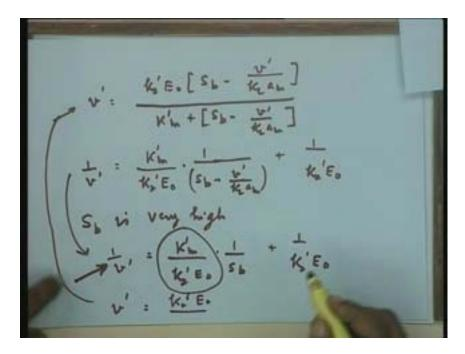
On the other hand when the substrate concentration is very low the slope will be  $1/k_l a_m + K^{'}_m/V^{'}_m$ .
