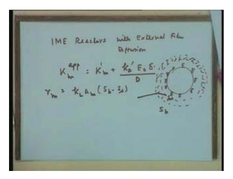
The rate of diffusion in such a situation let us assume the situation that this non-porous particle is packed in packed bed reactor and we operate it till a steady state is reached; steady state reached means the concentration of the substrate at the exit end becomes
