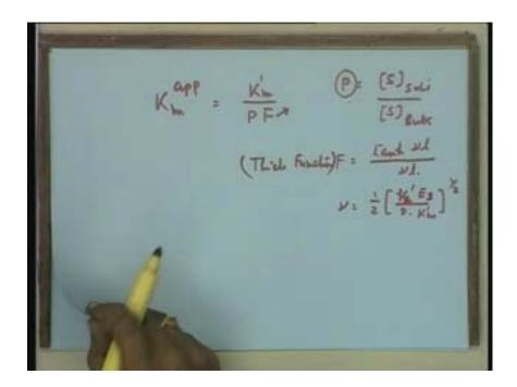
If you consider this function F that is  $\tanh \gamma l / \gamma l$ , the characteristics of this function is that when  $\gamma l$  is less than one that means in this region, the value of F is approximately equal to one. On the other hand when you go at  $\gamma l$  value greater than two F is approximately  $1/\gamma l$ .
