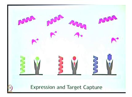
And these three proteins are going to get captured to the surface of the array because they have the GST tag. So, that is going to lock them down to their spot. But this does not have a GST tag. So, it is going to float everywhere on the across the array.
