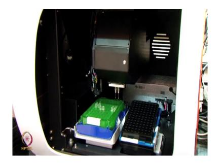
Now, this now the sensors are hydrated, I am going to place in the instrument the sensor holder, I am placing here like this. It should be firmly fixed in the group and now I am going to put the sample plate which contains the biotinylated antibody I am going to place like this in the sample plate. This is we call it as this particular part we call it as a sample compartment, this part we call it as a sensor compartments.
