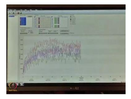
So, now this signal we are acquiring for the 30 seconds, that the first step we call it as a baseline. Now it is going to a next compart next column it is consists of a biotinylated protein A at 10 microgram per ml. Now we can able to see there is a rise in the signal this is what we call it as a immobilization step the biotinylated protein A is binding to the streptavidin sensor.
