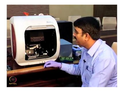
This is the Pall Forte Bio octet red 96 instruments. If we look at inside this is we call it as optical head box. The optical head box consists of a spectrophotometer as well as the channels or we call it as a manifold. This is 8 channel manifold.
