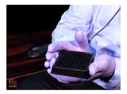
This is the plate map here this is the buffer the first column and the second column I am going to put the bio 10 microgram per ml concentration of a biotinylated protein A and the third column I am going to buffer with it you it will be useful as a for a unknown biotinaylated protein get washed off here and also this well I am going to useful for the dissociation purpose. And the last well, I am going to put the analyte that is a 25 microgram per ml serially diluted in a all these 6 wells.
