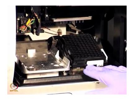
This is the sample plate 96 well plate I am going to place in the sample compartment here like this there is a clicks on it will come firmly it fits into the sample compartment. Here the sample compartment if you look at it is works on the dependent rate the BLI technology works on the dependent rate method here we do not have like a any micro fluidics devices.
