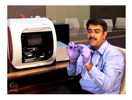
It is actually made up of the glasses consists of a fiber optic inside and the end at the holder part this is made up of the plastic. So, inside there is a fiber optic. At the tip of the sensor we are coating ligand of our interest. So, we are passing a white light. Light get reflected back, it is a reflection base phenomenon. One light which is coming from the internal optical layer another light which is coming from the ligand end.
