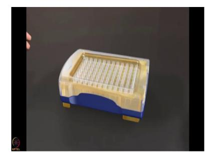
To disposable bio sensors measure binding events directly in a standard 96 well micro plate.
