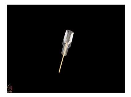
A proprietary protein coating at the tip provide reproducible coupling of target molecules in the minimum of nonspecific binding. Here we are using streptavidin coated sensors to setup a five step kinetic analysis with the first protein of the pair is biotinylated. (Refer Slide Time: 17:38)
