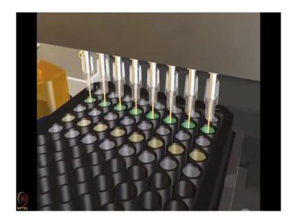
The streptavidin sensors are loaded by transferring into the wells with biotinylated protein. Bio layer interferometry is insensitive to change is in refractive index or PH of the matrix when more molecules binds to the streptavidin layer the optical thickness of the layer changes.
