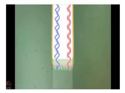
And as the thickness changes the interference pattern shifts. One nanometer of protein binding to the sensor produces a one nanometer shift to the blue in the interference pattern.
