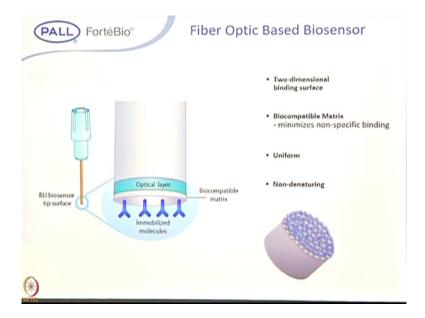
So, we are using a biosensor here as in the SPR they uses the chips the similar way we are using the biosensor here. The biosensor if you look at this is a sensor typically its looks like a needle, this is made up of a plastic and this is your a glass capillary which is nothing but the fiber optic. At the tip of this fiber optic we are coating a the biocompatible layer, it is a optical layer to that optical layer you are attaching a one of the protein of your interest.
