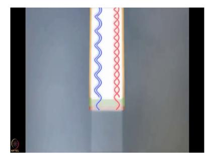
Most of the light scatters in a surrounding matrix. In a process that we call bio layer interferometry, the two reflections generate a spectro pattern rescollected and analyzed at the spectrometer. Constructive interference gives intensity peaks.
