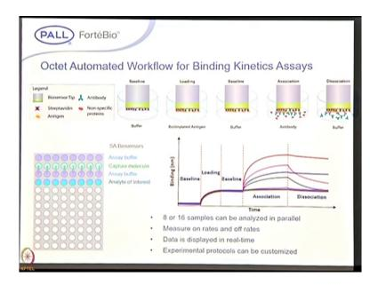
So, how exactly works the kinetics work flows? First the sensor will dip into the well containing a buffer you get a base line here and next we are till comes to dip into the well which have the loading. And then goes back to the well containing a buffer there exactly the unbound material get washed off and then corresponding analyte it is binding you can see the signal and the goes back to dissociation.
