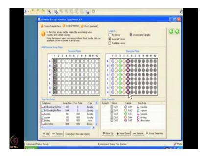
Up to 8 sensors can be run in parallel and the menu driven software assigns identities to each sensors to be used.
