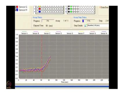
And the one nanometer change in optical thickness is recorded for that sensor in real time. The change in thickness related to the initial calibration is plotted for all 8 sensors.
