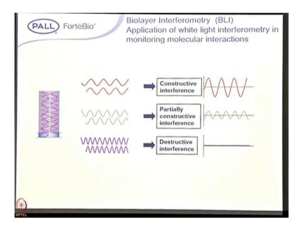
If you look at all this what exactly it is amplitudes different amplitudes we have, constructive interference, destructive interference this is what we exactly we plot relative intensity versus the wavelength. So, what happens?
