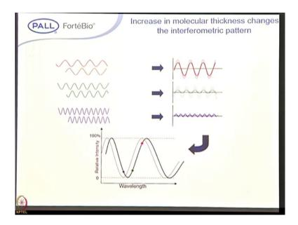
Once again if you look at all these waves are there earlier was the plot like this due to the molecules starts binding to the sensor surface you can see there is a shift in the interference pattern, this is what exactly as the molecule binds to the sensor surface you can see the shift. So, what happens exactly on the tip? The molecules bind to the sensor surface its forms a biolayer, its depends upon the thickness of the biolayer.
