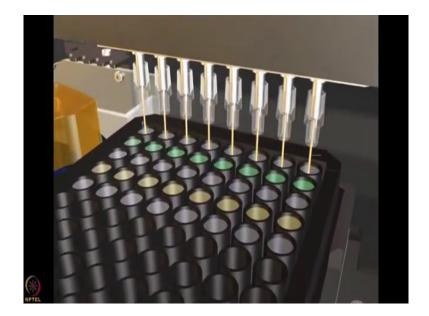
And the flow across the sensors surface is established to overcome mass transpose effects. Using optical fibers octet feeds broad spectrum white light down the sensor and collects the reflections.
