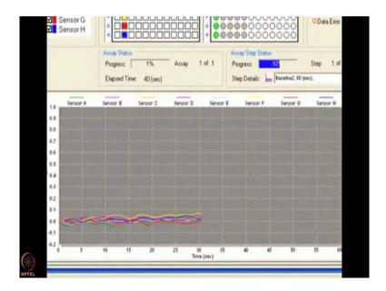
The position of the interference pattern is measured for all 8 sensors and then shifts in the pattern or plotted in real time.
