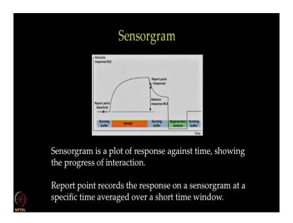
A sensorgram as shown here is a plot of response against time showing the progress of interaction. This curve is displayed on the system during the course of experiment. We observe the base lines followed by the injection of analyte which leads to increase in the binding response during the association phase.
