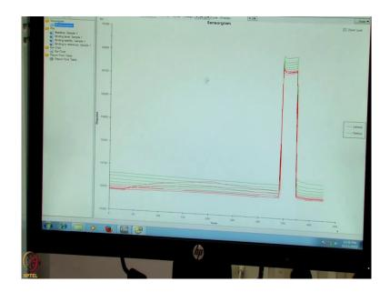
You can see here from our binding experiment which shows all sensorgrams here. So, here the green ones are our startups. So, we have setup 3 or 5 different startups, and the red ones are our actual data from beta 2 microglobulin.
