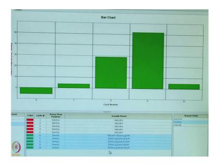
Here we will highlight the sample runs only and see cycle 7, 8 and 9 are our low, medium and high concentrations data which are dose dependent binding
