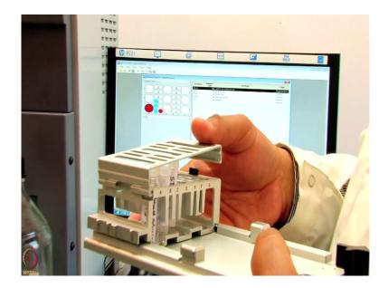
And we will fill it with the binding vials. So, these vial positions are filled with different samples. As you can see on the screen the startup is here. So, beta 2M medium, beta 2M low, beta 2M high are put at their respective positions and a vial for regeneration of 10 millimolar glycine pH 2.5 is here. Now, we close the rack and will be inserted in the sample compartment by ejecting the rack compartment, inserting the plate. Next tab.
