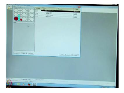
Here we have at the C one position HBSEP plus buffer for 3 different startups. We have 3 concentrations of analyte, high, medium, and low, and we have the regeneration solution here which is 10 millimolar glycine pH 2.5. And we will prepare our solutions and start the binding experiment.
