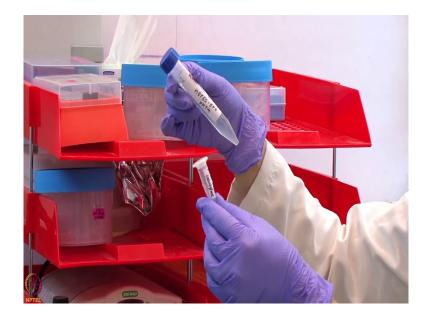
We then dilute the stock solution of protein that is 100 microgram per ml in the running buffer HEPES EP plus.
