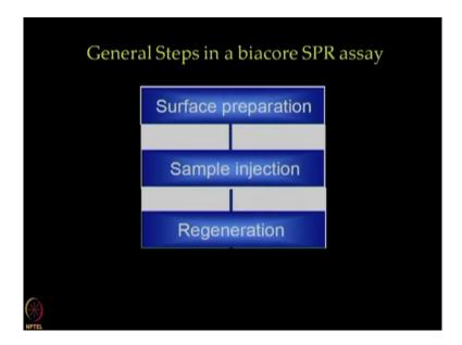
The three major steps in a biacore, SPR assay involve immobilization, the process by which ligand is attached to the sensor chip surface; interaction analysis, where the analyte is injected over the sensor chip surface and the interaction between the analyte and the immobilized ligand is monitored and regeneration, the process of removing bound analyte from the ligand on the surface.
