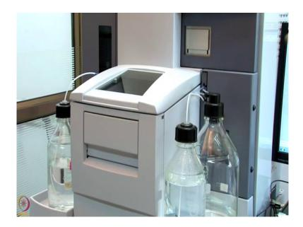
So, this is a surface plasmon resonance and it is a Biacore T 200. So, this machine has the various parts like, the running buffer is connected here and any of the biological buffers can be connected as a running buffer. They could be have any pH from low to high. So, the regular buffers used in a biacore experiment are HBS EP-HBSN PBS for small molecule experiments.
