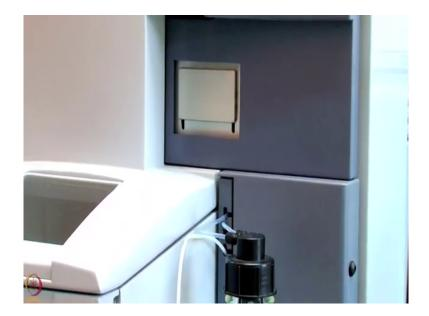
This chip will be inserted in the chip docking area. From the control software, we will eject the sensor chip that is connected.
