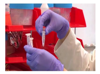
Aliquots of NHS, EDC and ethanol amine are prepared and transferred to the specialized tubes used for the system.
