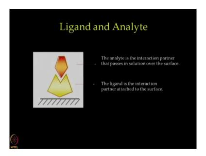
Let us learn a little about the basics of immobilization and SPR assay. In the molecular interaction study using surface plasmon resonance, we will immobilize one of the interacting molecule that is anti beta 2 microglobulin on the gold sensor chip surface; while the protein beta 2 microglobulin will be passed over that surface in solution
