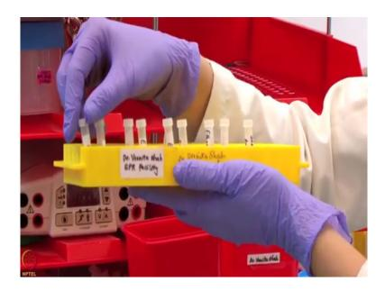
We have now transferred all the reagents into these specialized tubes. So, we have two NHS tubes, two EDC, two empty tubes for longer stability of EDC, NHS which will be mixed inside the system; two ethanol tubes, one for the blank flow cell and the other for the active flow channel and one ligand solution.
