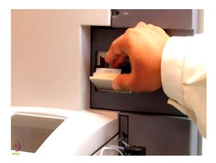
So, now the old chip will be removed and we will insert a new biacore chip CM 5 here. And the insertions or the way orientation of the chip is shown on the chip in arrows. And we will close the compartment door and identify the chip from the chip type here.
