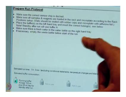
So, here there are some points we need to take care before start of the run. Make sure the correct sensor chip is docked, make sure all sample regents are loaded in the rack and microplate according to the rack position set up. Vials should be sealed with caps, place the buffer, place water and make sure there is sufficient amount of water and buffer.
