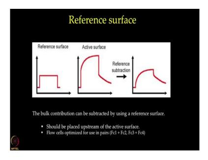
Reference subtraction is particularly important for assays, where measurement is taken during the sample injection. The bulk contribution due to any difference in the sample matrix and running buffer can be subtracted by using a reference surface. This reference surface is typically placed upstream of the active surface. The flow cells on the chip surface are optimized accordingly for use in pairs that is flow cell 1 with flow cell 2 and flow cell 3 with flow cell 4.
