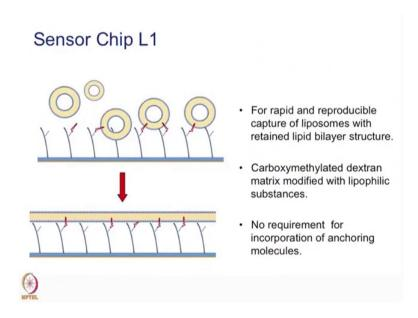
L 1, another surface sensor chip which is also popularly used for studying liposomes, lipid bilayer kind of a molecules and carboxymethylated dextran is modified with lipophilic substances.
