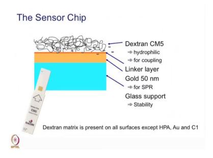
If you look at a particular gold surface on a chip, it contains a layer of dextran and that dextran provides or supports the interaction or immobilization of your ligand on the chip. The dextran is glued to the gold and the gold is present in form of a cassette and that cassette entirely is called as chip. So, looking into this gold surface the major component attached into the gold surface is the dextran and it is very important for us to understands why dextran.
