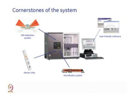
So, the corner stones of any SPR system or a Biacore system is a detection system and a chip system, a micro fluidic system and the software which integrates all of these and generates data. So, in our next sessions and next couple of other sessions we will anyway understand details about sensor chips and the different sensor chips available that the SPR detection system depends upon the in refractive index, and also depend upon the surface concentration and temperature.
