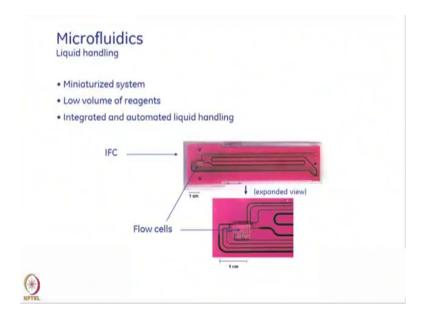
The interactions happen in a miniaturized system called micro fluidics which are the liquid handling part of the system, which contains very low volume of reagents and they are integrated and automated liquid handling systems where the flow cells are actually situated and the actual interaction happens and recorded by the system.
