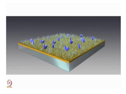
A glass slide coated with a thin gold film creates the sensor surface. For most applications a dextran may discovering the gold film acts as a substrate to which molecules can be attached and provides a hydro silicon environment for the interaction. Other mattresses can be used to attach specific types of molecules. The specificity of the surfaces is determined by the nature of the molecule attached to it.
