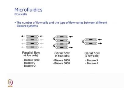
There could be many ways of orientation of the micro fluidics and the flow cells. It could be a parallel way, a serial way or a two cells at a time and different systems can have a different way of the fluidics and also different orientations.
