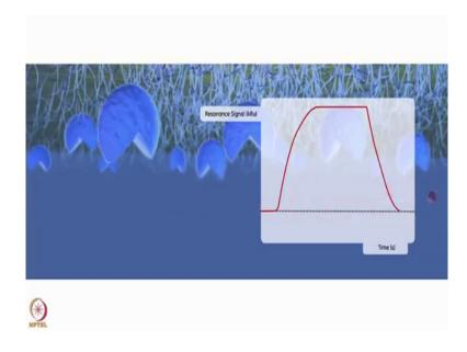
The sensor surface, the micro fluidic system and the SPR detection unit worked together to measure bimolecular interactions. The result from the detection of change in refractive index is displayed as a sensor ground with the binding response on a wide axis is plated against time in the x-axis. Since, light is not penetrate the sample analysis can be performed on colored turbid or opaque samples.
