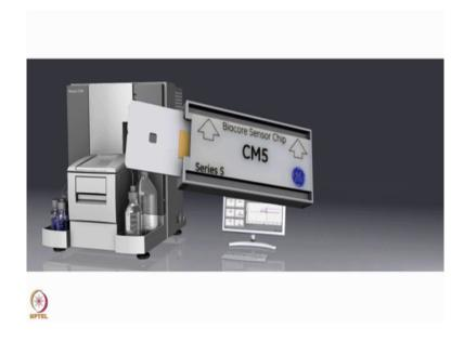
In Biacore systems molecular interactions or monitored under a movable sensor chip by the Surface Plasmon Resonance detector.
