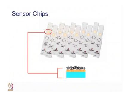
So, the various chips that are available for any SPR experiment to start with they are named as CM 5 chips, CM 4 chips, CM 3, C 1 streptavidin or an SA chip, NTA chip, L 1, HPA and Au or a plain gold surface chip. Each of this chips have a place for an adapter and this adapter actually holds the gold and that gold applies is where the immobilization happens and the adapter actually pushes the gold surface in to the SPR system where actually immobilization happens.
