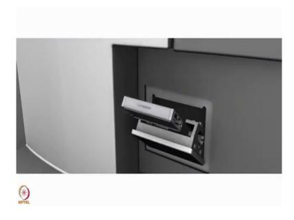
Samples and reagents are held in removable racks and are delivered the chip by micro fluidic system that uses a very low volumes of sample down to a few micro liters.
