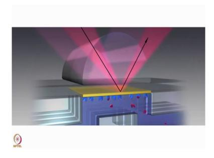
Biacore uses the phenomenon of Surface Plasmon Resonance to detect bio-molecular interactions as they happen. SPR causes a reduction and the intensity of life reflected at a specific angle from the glass side of the sensor surface. As molecules buying to the sensor surface the refractive index close to the surface changes, altering the angle of minimum reflected intensity. The change in SPR angle is proportional to the massive material bound.
