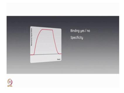
From studying the shape of the sensor ground produced binding yes or no specificity, affinity, kinetics and active binding concentration can be determined. The sensorgram provides real time information about the entire interaction.
