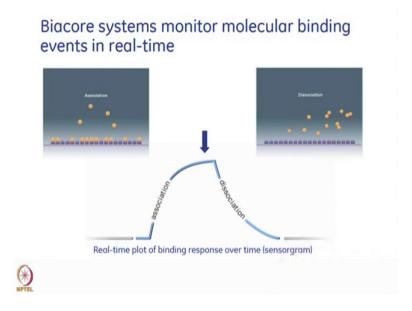
So, basically experiment starts with an immobilization of a ligand on the sensor surface and an analyte is passed over in a solution and which will bind to the ligand. So, here they are two different molecules, one of them is ligand and analyte and the interaction is recorded in a real time and the data that is output on the surface.
