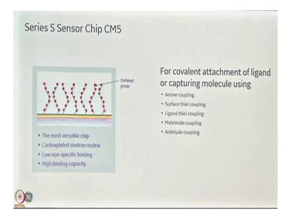
So, you know the basic structure of the chip. The chips are actually on the glass surface on which there is a gold coating, then there is a linker molecule where the dextran molecules are stuck to it and the dextran molecules have carboxyl methyl groups. And in these carboxyl methyl groups is where your covalent linking happens ok. The CM 5 chip is actually our most versatile chip you know any.
