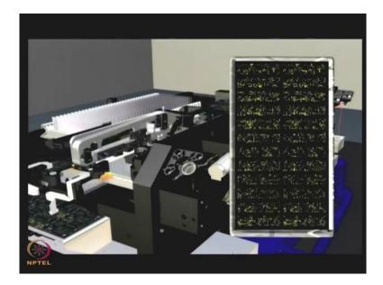
Each channel is scanned sequentially and the developing images are displayed on the monitor.
