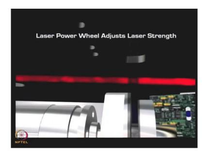
A neutral density filter wheel can be used to attenuate the laser power if necessary for especially bright samples.
