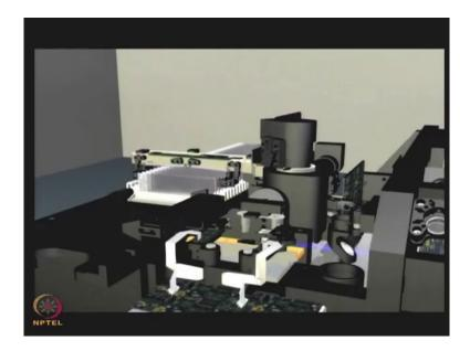
After the slide has been scanned the precision robot arm replaces it safely in the slide carrier before picking up the next slide.
