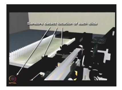
As the carrier is inserted into the scanner sensors detect the location of each slide indicated by a blue bar on the slide carrier map.
