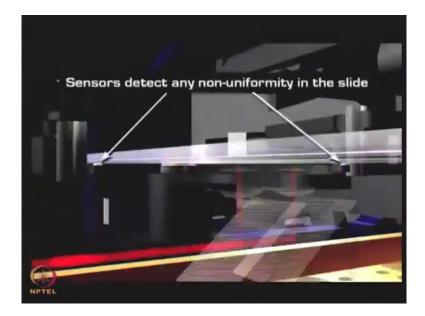
Fluorescent signal emitted from the sample is collected by a photomultiplier too. As the scam proceeds sensors detect any non-uniformity in the slide surface.
