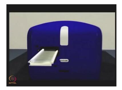
As many as 36 slides can be loaded into the convenient slide carrier.
