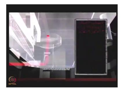
The beam scans rapidly across the short axis of the slide as the robot arm moves the slide more slowly down the long axis.
