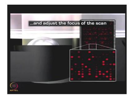
And, the robotic arm adjusts the slide position accordingly to ensure the array surface is always in perfect focus.
