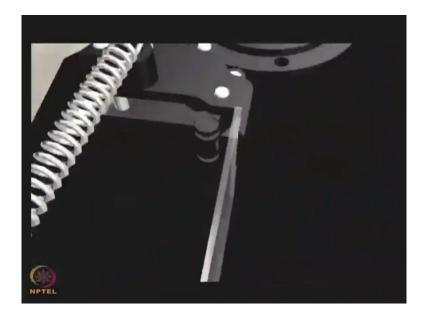
A unique never let go rippers securely clamp the slide and carry it to the scanning area. A barcode reader records the barcode and then the slide is positioned for scanning.
