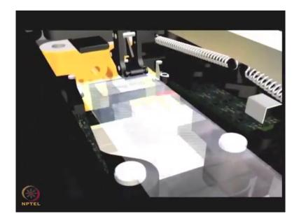
The laser excitation beam is delivered to the surface of the microarray slide.
