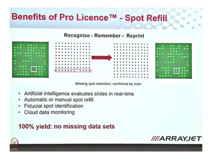
So, it is an artificial it is actually a part of artificial intelligence software, which evaluates your slides real time. It is automatic or manual spot refill and it provides 100 per cent yield no missing data sets. So, there is no need to repeat your experiments for a whole month. So, it remembers that there is something that is missing here and what it does the next time you have a spot here.
