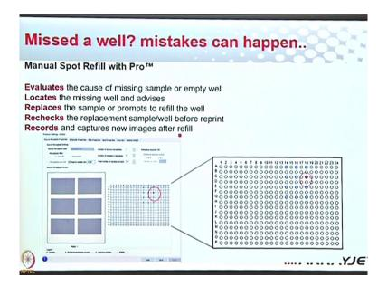
So, there are spot refill features. Now spot refill means you can reprint that spot wherever it is a missing place, it will go and put your sample. So, it evaluates the likely cause of the missing sample. Sometimes what happens if air goes inside or you have forgotten to fill a well because these are 3 8 4 well plates.
