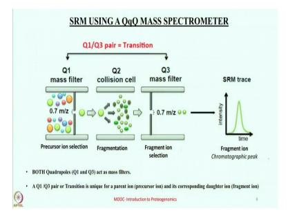
So as you can see from the slide, selected reaction monitoring uses a triple quadrupole mass spectrometer and in this current slide we can see that there are three quadrupoles quadruple 1
