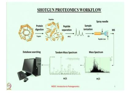
I am sure that by now you are very well acquainted with the steps involved in a shotgun experiment, but I would quickly walk through the major steps that are involved. So, we start with say the protein lysate on which the experiment is to be performed and then using a protease, we digest these proteins to give rise to peptides. The digested peptides are then separated on column and using electrospray ionization, the peptides get charged.
