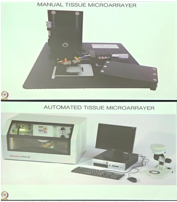
use more sophisticated tissue microarrayers that are automated, automated microarrays can make up to 20, 25, 30 microarray blocks a day, but it's an instrumentation which has its own problems, so if you don't have that workload it's not nothing to get into, you're much better off with the manual microarrayer.
