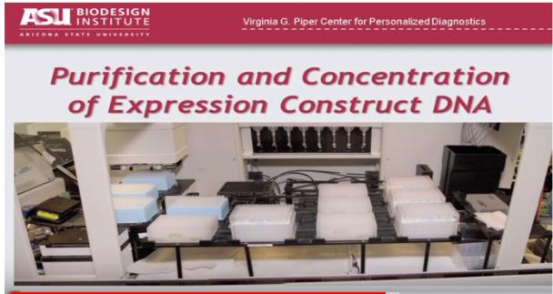
Lysate is loaded directly into the DNA binding plate using the Biomek FX
