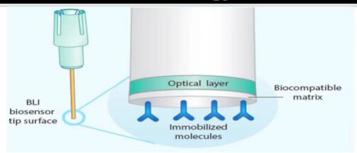
Analyses interference pattern of white light reflected from two surfaces, ligand at surface of the tip & an internal reference layer.
