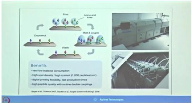
So this has 24 different nozzles, because 20 amino acids are there, and so we have 24 nozzle and 20 amino acid + 4 is to de-protect basically, so how we do, so we directly synthesized this peptides on the slide, so this is 20 nozzles so basically adding amino acid at that synthesize on the top and deprotect it, so one by one you can synthesize 15 or 20 based peptide or 30 based peptide according to your requirement, right.
