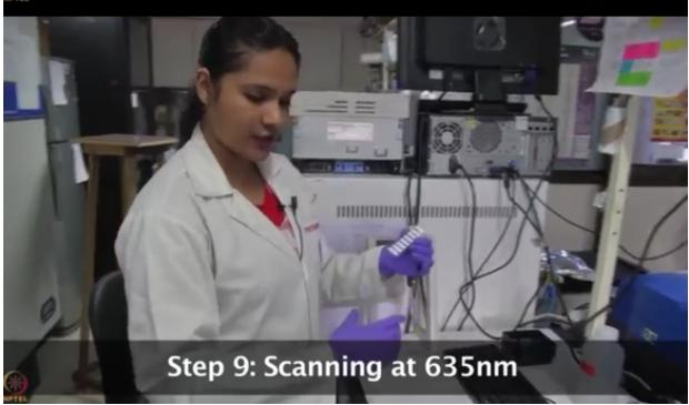
So we're going to now scan the slide as you will see the slide is dry after centrifugation, we will place the slide carefully in the scanner with the barcode side facing downward, so now we'll scan the slide.
