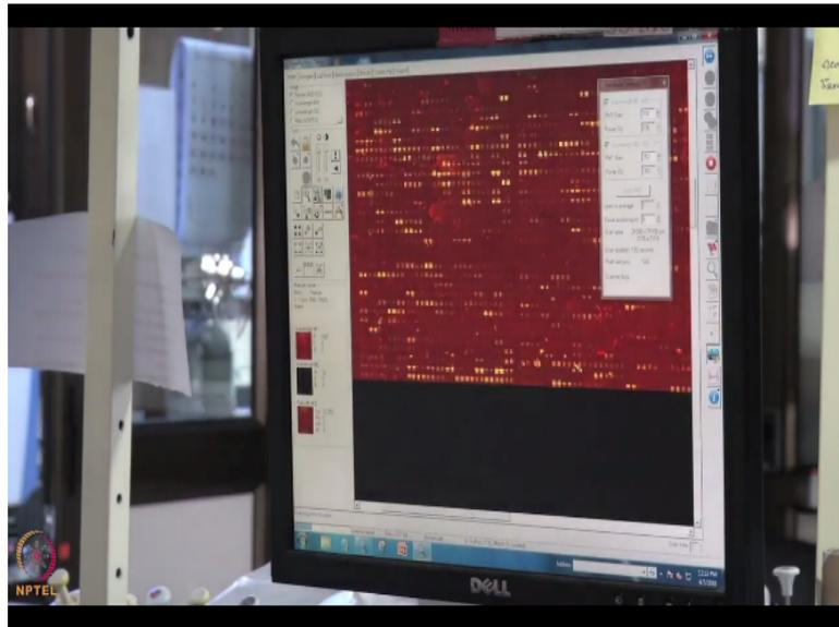
Now if I increase this also to say 600, then you can see that the whole intensity is increasing. So PMT's parameters are very important because when you have to scan a slide, all the spots should be scanned at a particular wavelength and you do not want to miss out on a lot of spots as well as you do not want most of the spots to be saturated. So auto PMT is one of the options where you can go and it will just scan the slide at 3 different wavelengths.
