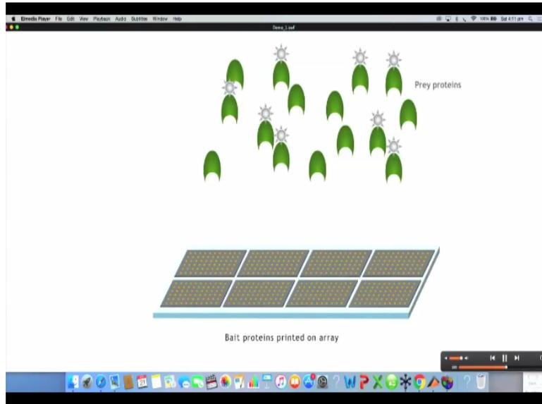
Protein microarrays are widely used for protein interaction studies. One of the proteins to be analyzed is printed onto a microarray surface usually made of glass. The proteins known as bait proteins get immobilized onto the array surface that is functionalized with reagents like nickel or aldehyde compounds that interact with groups present in the protein. This bait protein is then probed for interactions with suitably labeled query or prey proteins.
