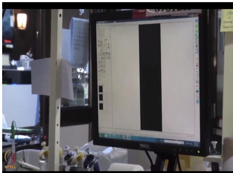
So what you do is you set the wavelength because it is a dual-channel thing, you set it for red channel, we set it at 635 nanometers. For green channel, we set the wavelength at 532 nanometers and then we go for the PMT settings. So usually if we keep PMT settings at red channel at 500 PMT gain 100% laser power and PMT gain at 350. This settings you can optimize using auto PMT.
