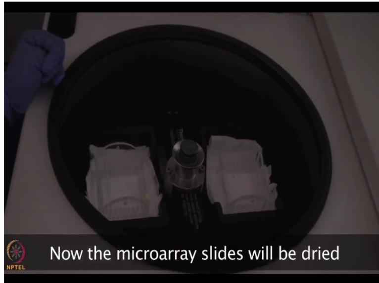
So once you keep the slide, close the lid and here the parameters are speed is 900 Rpm, time is 2 minutes, acceleration and deceleration is 8 and 8 and the temperature is room temperature. So once you keep the slides then spin it. So just you have to start the spinning. So after centrifugation now we are going to take out the slides. So you can see now the slide is completely dry.
