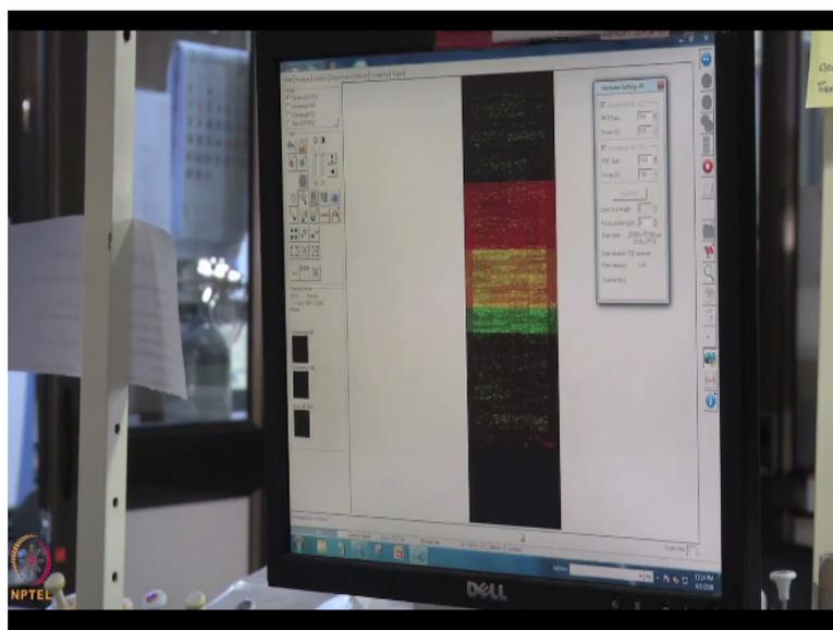
So this is how the preview scan looks like. So once you have done it, you can just lay over the grid like the way you put you set an area for your paper scanning, you can set the area for scanning of the slide, so if you want only this much of area to be scanned, you can just resize
