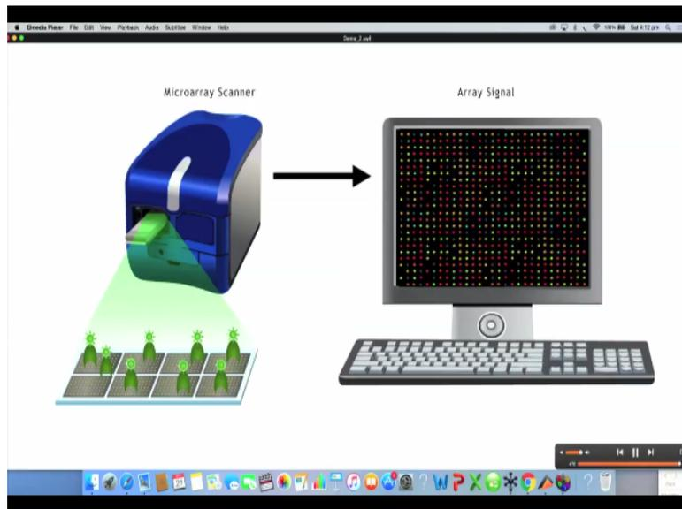
Once the unbound proteins are washed off the array surface, the protein interactions are detected by means of an array scanner. These protein microarrays are extremely useful in studying interactions with other proteins as well as small molecules DNA or RNA. Let us now talk about a different type of protein microarrays platform. For example, the direct labeling based method.
