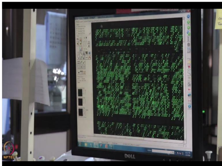
This is how in green channel the slide looks like and green channel is majorly done for checking the quality of the slide, for checking the printing quality of the slide. So now if you
