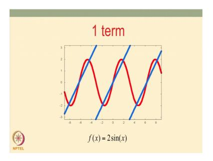
I take one term by one term and plot, if I take the first term which is 2 sin x, I plot the saw tooth function is in blue and the first term is red.
