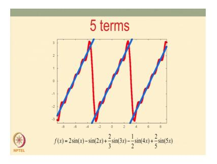
If I add 5 terms. So, these are the 5 terms described below these are the 5 first 5 terms of that infinite series. So, write down these infinite series and check if these are the 5 terms of their infinite series you would get this nice saw tooth like function.
