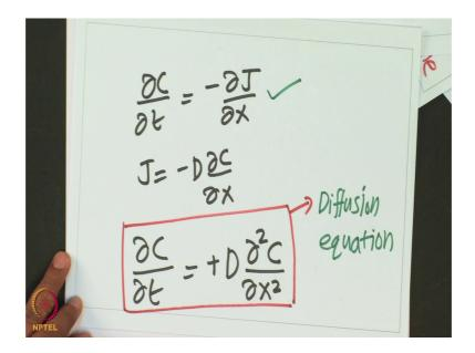
I will get that del C by del C by del t is equal to minus del J by del x J is equal to minus D del C by del x I substitute this J here I will get del C by del t is equal to minus D and there is a minus. So, it will become plus plus del square C by del x square.
