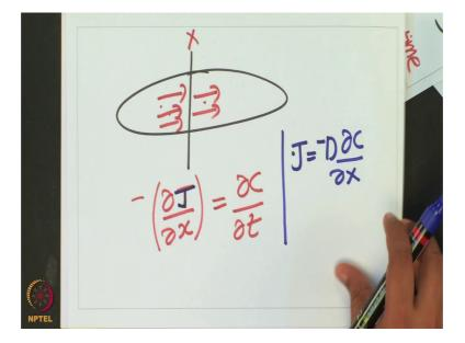
You look at the flow that is coming in and the flow that is going out. So, J here and J here this del J by del x depending on this value of del J by del x if the del J by del x is 0
