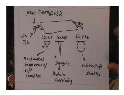
So, if I were to draw an AFM. So, what you have. So, these are tips. So, this is called a AFM cantilever, and this is called an AFM tip it is called an AFM tip. So, you can have various geometries of these tips. So, for example, if you want to image something your tip so, if I were to just draw the tip geometries. You can have tips which are very sharp, you can have this is let us say a blunt tip. You can have a very sharp tip or you can have the tip is nothing but a spherical ball sphere ok.
