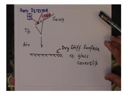
Now, let us see how does the cantilever operate. So, you have you have this is the AFM tip. And what is done so, the backside of this, this is shiny. So, you have a laser which focuses at this point. You have a photo detector and you send a laser light, which focuses on the back of this cantilever and reflects of the back and gets detected by a photodiode photo detector. So, for example let us assume that tip is trying to probe this particular substrate which can be just glass.
