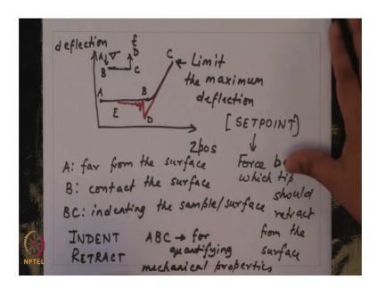
So, if I were to draw a complete cycle, a complete cycle. So, let us say this is z position and this is deflection. So, you generate so, this is a curve that you get as raw data from an AFM experiment. So, let me label some points, at point A you are far from the surface, at point B you contact the surface. So, in B to C you are indenting the sample or surface.
