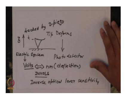
So, when it comes and touches the surface. So, you have deformation of the tip. So, and this deformation is what is tracked by the photo detector. So, any what is detected in the photo detector is in volts ok.
