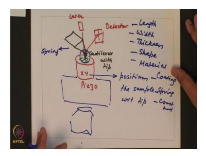
So, this cantilever acts like a spring and you have the sample which is resting on an X, Y Piezo. This whole setup is mounted on an inverted microscope. So, you have your objective below.
