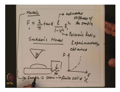
So, what you do is you fit these curves to various models. There are various models where you have a given profile. So, of in order to extract the stiffness value from the raw data you use various models; for example, this is one model. So, this model is called a sneddons model. This is applicable when you have a conical tip which is indenting your sample.
