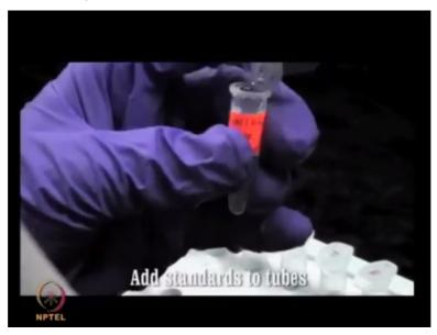
Add an increasing concentration of standard protein sample to each of the designated tubes. Bovine serum albumin is often used as a standard. Then add the unknown protein sample whose concentration is to be determined to the appropriately labeled tube. Dilute all the samples uniformly using the sample buffer.
