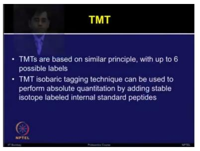
I have given you the reference for the original study on tandem mass tag in the slide. So these tandem mass tags they are based on the similar principle of iTRAQ. Here the possibility for multiplexing is up to 6 possible labels. The TMT isobaric tagging technique can be used to perform absolute quantification by adding a stable isotope labeled internal standard peptides.
