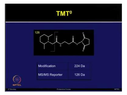
The TMT 0 tag is used for testing and optimization of sample preparation, labeling, fractionation and MS fragmentation for peptide identification and reporter detection. The modification is 224 Daltons and MS/MS reporter ion is 126 Daltons.
