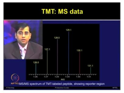
I am sure (()) (26:29) representative MS/MS spectrum of TMT labeled peptide, which is showing a reporter region. The relative abundance of target protein or peptide fragment in such different samples can be easily measured by comparing these signature mass peaks, which are generated by the different mass tags.
