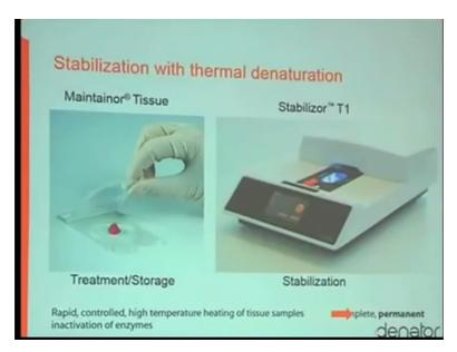
So this is the problem that we are addressing and to do this we stabilize through thermal denaturation. So we use heat, a heat based technology and in the next slide I will show you exactly how it is done and what happens on a molecular level. So we have the instrument itself, there is a cartridge, this is the cartridge for solid tissue, there is a cartridge for liquid samples. There is also a cartridge for DBS, dried blood spots.
